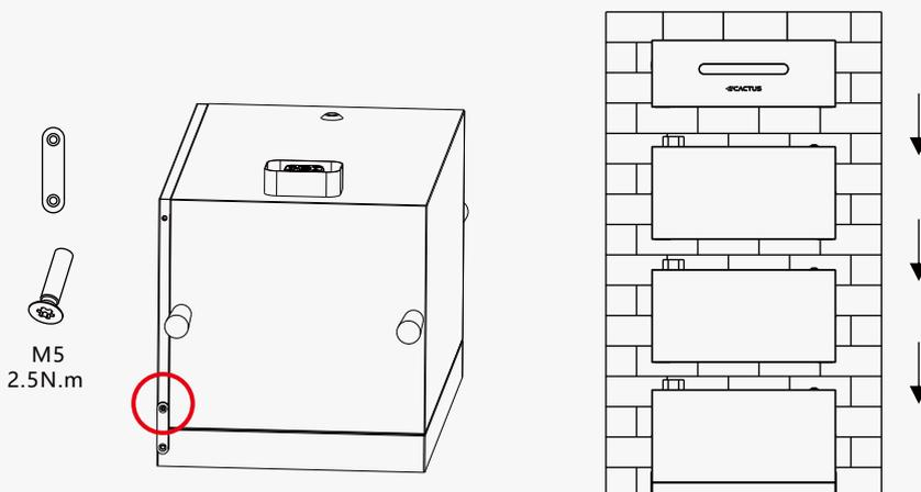
\*Please secure the connecting plates at each battery box before stacking them and use lifting equipment when installing the sixth battery box.
