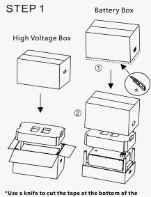
\*Use a knife to cut the tape at the bottom of the battery box and pull it upwards to separate the top carton and the base carton.
