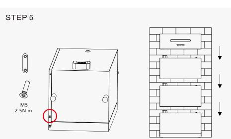
\*Please secure the connecting plates at each battery box before stacking them and
